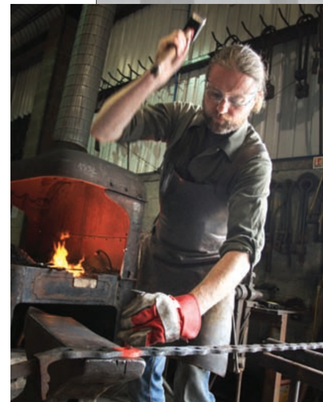
Arek hot punching holes in wrought iron for a new gate
