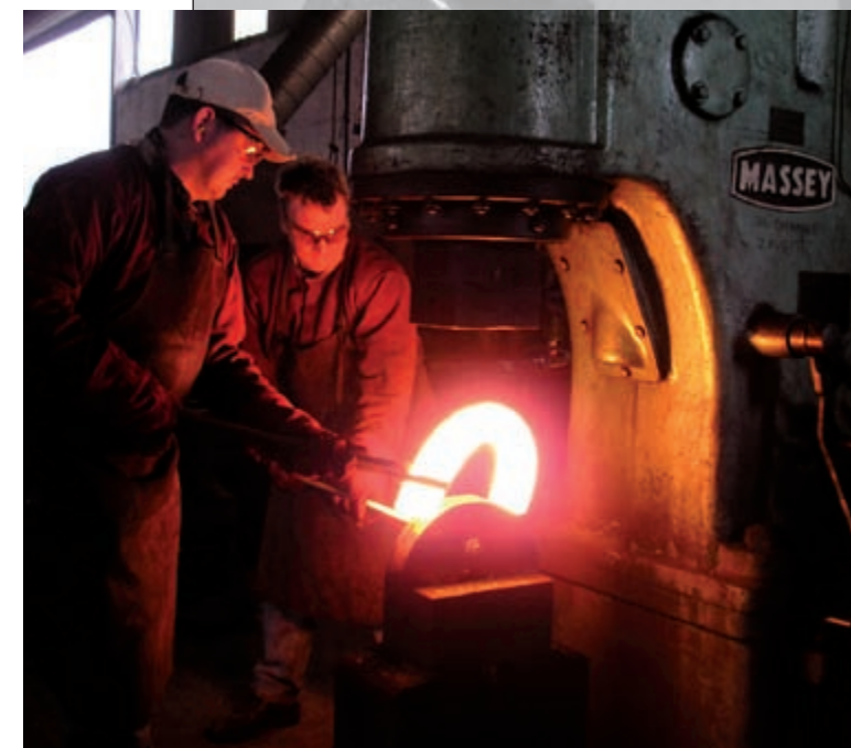
Straightening a chain link under the hammer before rolling
