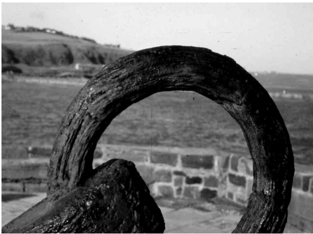
Grain structure on an old ships anchor
