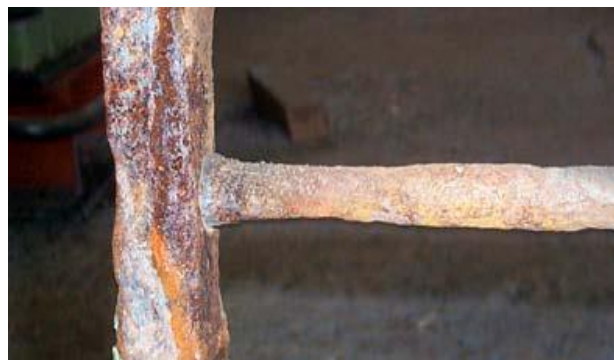
Arc welded insert-mild steel
