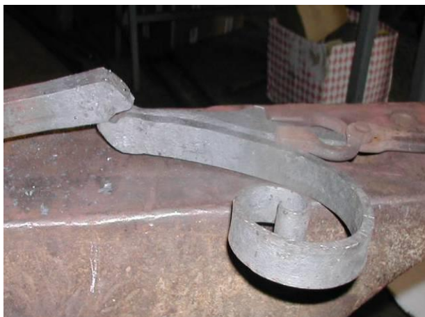
Preparation of joint for forge welding
