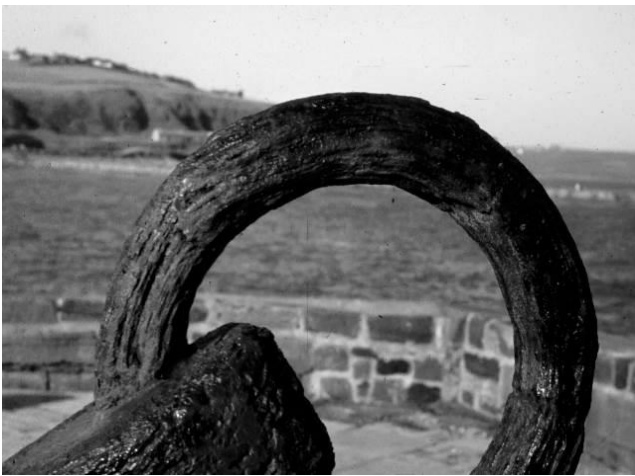
Grain structure on an old ships anchor
