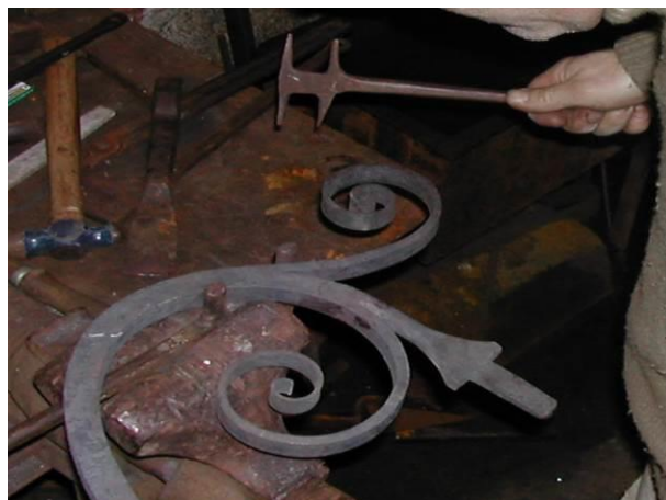
Shaping finished branch welded scrolls
